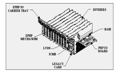
Figure 2-12: I/O Carrier Tray
